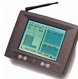
The TRAQ Manager clamp truck runs Windows applications that provide the operator with information such as: order status, production plans, inventory, and vehicle availability. The clamp truck workstation is a mobile decision-making tool, empowering the driver to make informed decisions about roll storage, loading and other inventory-management issues.
